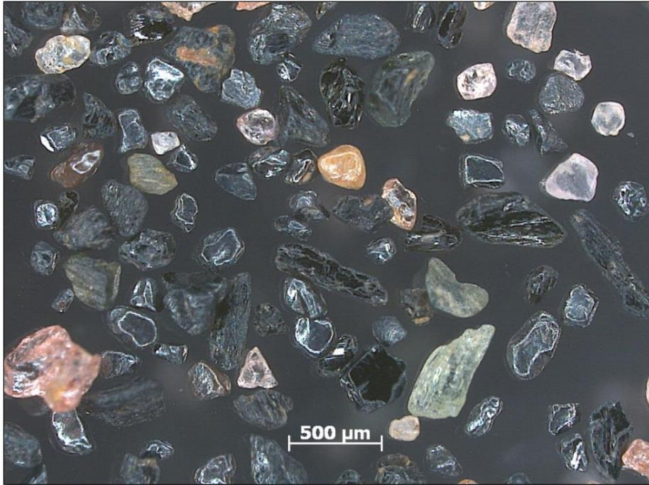
**Figure 12:** Stereomicroscopic image of a magnetic-others fraction.
