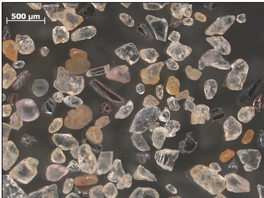
**Figure 13:** Stereomicroscopic images of a non-magnetic fraction.
