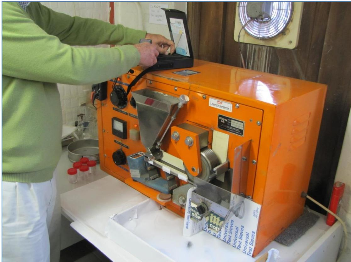
**Figure 9:** The CARPCO high intensity magnetic separator.
