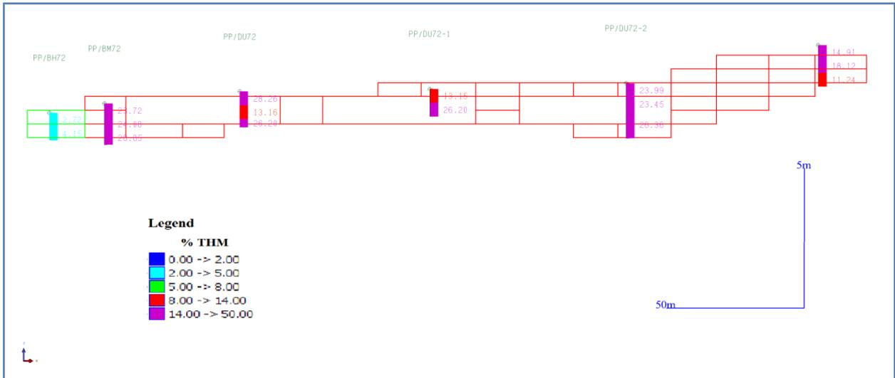
**Figure 14:** Section on EL180 on Mannar showing the input drillhole values of the % THM correlate well with the block model estimates. Vertical exaggerations 10X.
